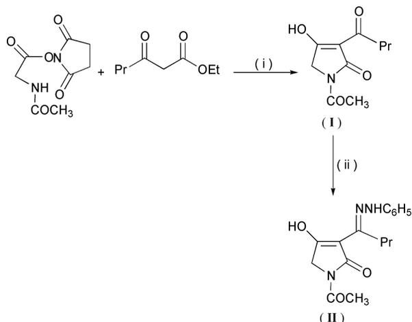
**Scheme 1** Synthesis of the ligand Habta **I** and its phenylhydrazone derivative **II**. (i) NaH, PhH, r.t.; (ii) H<sub>2</sub>NNHC<sub>6</sub>H<sub>5</sub>, abs. ethanol, reflux 2.5 h.
