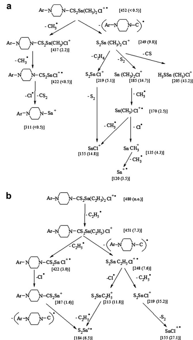
Fig. 2. Proposed fragmentation patterns for (a)  $\text{Me}_2\text{SnCl}(\text{MPPDA})$  (**1**) and (b)  $\text{Et}_2\text{SnCl}(\text{MPPDA})$  (**2**); [mass(% of the total positive current carried by identified tin-containing ions)].
