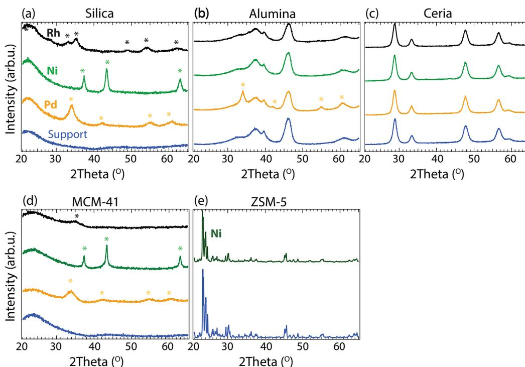
**Fig. 1** X-ray diffraction patterns of the support materials (blue) and as-prepared Pd (orange), Ni (green) and Rh (black) catalysts (3 wt.%) supported on a) silica b) alumina c) ceria and d) MCM-41. e) shows the XRD pattern for 1.5 wt.% Ni (dark green) ion-exchanged into ZSM-5.
