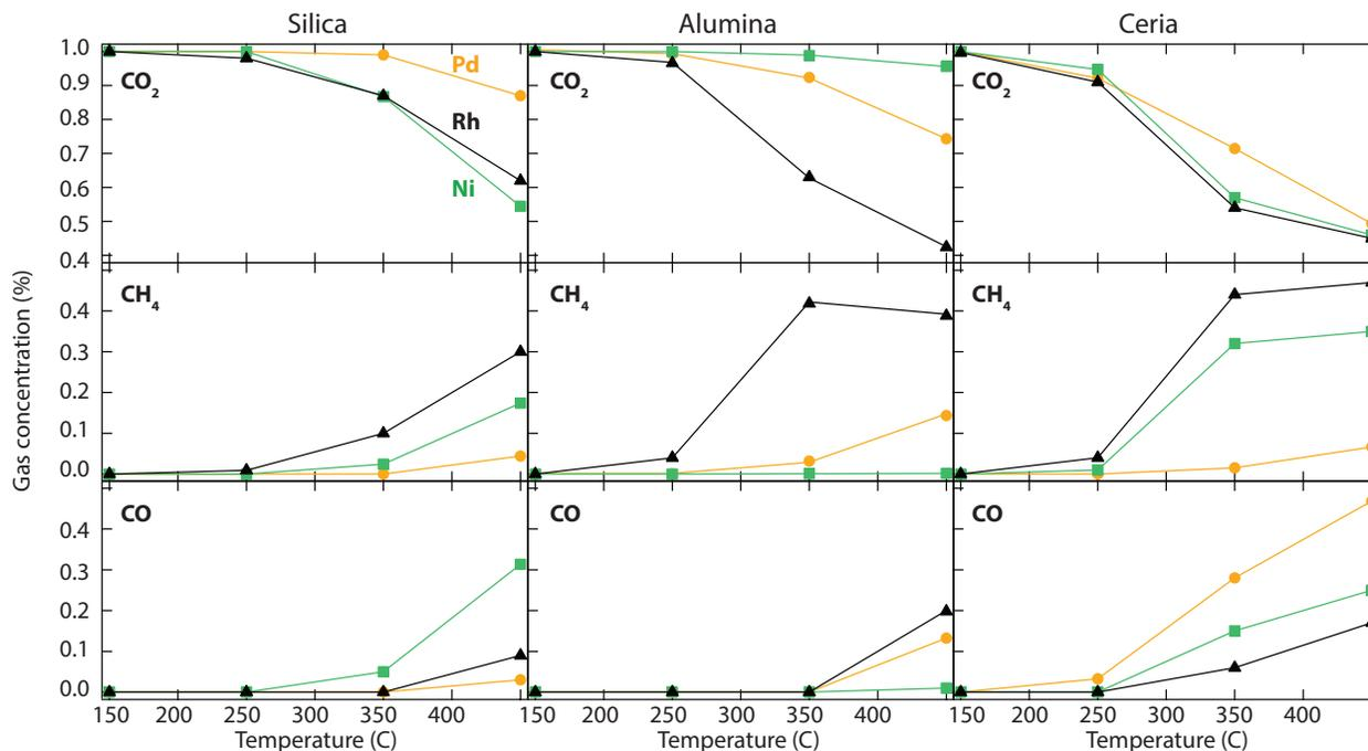
**Fig. 2** Steady-state outlet concentration of CO<sub>2</sub> (top), CH<sub>4</sub> (middle) and CO (bottom) as a function of temperature during the reaction between 1% CO<sub>2</sub> and 5% H<sub>2</sub> in Ar between 150 and 450 °C at a total flow rate of 2000 ml/min at atmospheric pressure over the silica, alumina and ceria supported Pd (orange), Ni (green) and Rh (black) catalysts.
