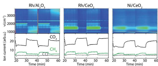
TOC: CO<sub>2</sub> methanation over Rh/Al<sub>2</sub>O<sub>3</sub>, Rh/CeO<sub>2</sub> and Ni/CeO<sub>2</sub> at 350°C highlighting the different surface speciation during reaction.
