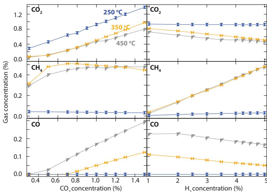
**Fig. 3** Steady-state outlet concentration of CO<sub>2</sub> (top), CH<sub>4</sub> (middle) and CO (bottom) over Rh/CeO<sub>2</sub> as a function of inlet concentration of CO<sub>2</sub> at constant H<sub>2</sub> concentration of 5% (left column) and as a function of inlet concentration of H<sub>2</sub> at constant CO<sub>2</sub> concentration of 1% (right column) in Ar gas with a total flow rate of 2000 ml/min at atmospheric pressure.
