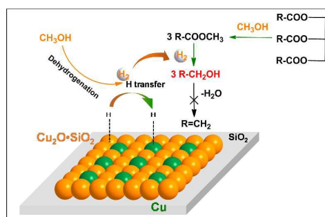
Fig. 6 The designed reaction pathway for Cu/SiO 2 -HT catalyzed selective conversion of coconut oil to fatty alcohols in methanol. Reaction conditions: coconut oil (0.3 g), Cu/SiO 2 -HT (0.2 g), methanol (40 mL), 240 °C, 4 h, stirring at 400 rpm.
