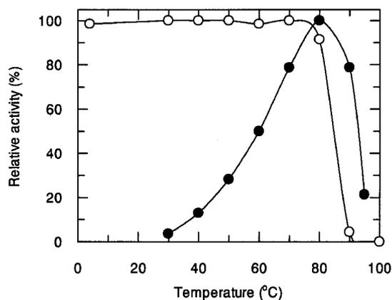
Fig. 2. Temperature Stability and Activity of Agu4B.
