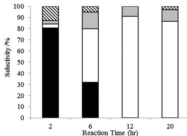
Fig. 2 Selectivity to DHMF (black), DHMTHF (white), polyols (grey) and unidentified products (striped) as a function of reaction time for the hydrogenation of HMF over Ru/CeO<sub>x</sub>.
