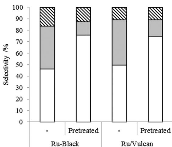
**Fig. 4** Selectivity to DHMTHF (white), polyols (grey), and unidentified products (striped) in the hydrogenation of HMF over Ru-black and 1 wt% Ru/Vulcan without and with feed pretreatment with Amberlite IRA-400(OH).
