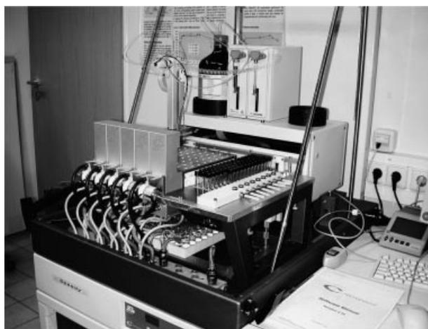
**Figure 4.** Chemspeed ASW 2000 Synthesizer.
