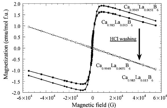
Fig. 1. Magnetic field dependence of the magnetization of  $\text{Ca}_{0.9949}\text{La}_{0.0051}\text{B}_6$  (closed circles) and  $\text{Ca}_{0.985}\text{La}_{0.015}\text{B}_6$  (closed squares) at 300 K, and the magnetization of HCl washed  $\text{Ca}_{0.9949}\text{La}_{0.0051}\text{B}_6$  (open circles) and  $\text{Ca}_{0.985}\text{La}_{0.015}\text{B}_6$  (open squares). The data for  $\text{Ca}_{0.9949}\text{La}_{0.0051}\text{B}_6$  is the same as that given in Ref. [6].
