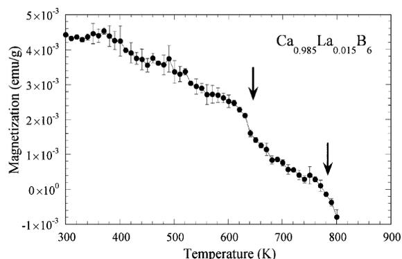
Fig. 3. Temperature dependence of the magnetization of  $\text{Ca}_{0.985}\text{La}_{0.015}\text{B}_6$  measured with a field of 1 kG. The arrows indicate the anomalies observed at 640 and 780 K.
