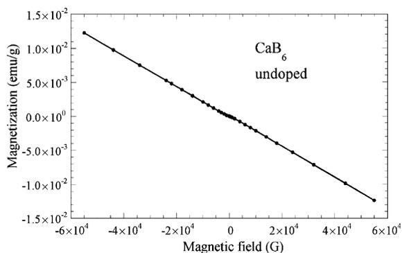
Fig. 2. Magnetic field dependence of the magnetization of undoped  $\text{CaB}_6$  at 300 K.
