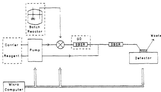
**Figure 1.** FIA manifold for investigation of mutarotation kinetics. Hatched lines indicate thermostated components.
