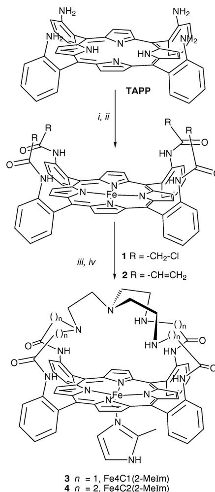
**Scheme 1** Reagents and conditions: (i) chloroacetyl chloride or acryloyl chloride in dry THF-NEt<sub>3</sub>; (ii) FeBr<sub>2</sub>-THF-2,6-lutidine under nitrogen; (iii) TREN in THF or MeOH at 55 °C; (iv) 1000 equiv. 2-methylimidazole.
