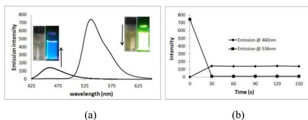
**Figure 1.** (a) To 5  $\mu\text{M}$  probe **1** in DMF was added 100  $\mu\text{M}$  DCP, the emission spectra was recorded every 30 s over 150 s. The inset picture showed the color change and the fluorescence change under a UV lamp. (b) The fluorescence intensities at 460 and 536 nm vary in a time range of 150 s. The excitation was set at 410 nm with slit/slit 5/1.5.
