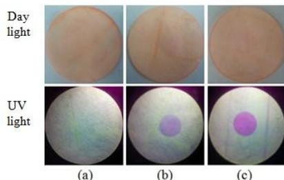
**Figure 3.** (a) Filter paper treated with 0.1 mg/mL probe solution in MeOH in the presence of  $K_2CO_3$ . (b) Filter paper exposed to DCP vapor for 1 min. (c) Filter paper exposed to DCP vapor for 5 min. Pictures at the bottom was irradiated at 365 nm with a UV lamp. Filter paper was used.
