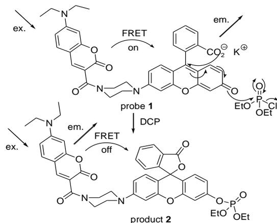
**Scheme 2.** Design of FRET-based ratiometric fluorescence probes for OP nerve agents.
