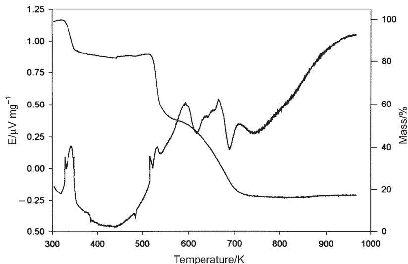
Fig. 6 TG and DSC curves of 5-chloro-2-methoxybenzoate of Mn(II)
