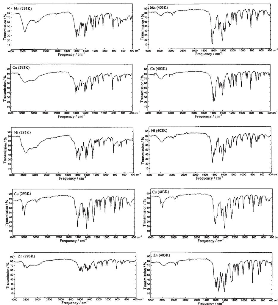
**Fig. 2** Infrared spectra of 5-chloro-2-methoxybenzoates of Mn(II), Co(II), Ni(II), Cu(II) and Zn(II) at 293 and 403 K
