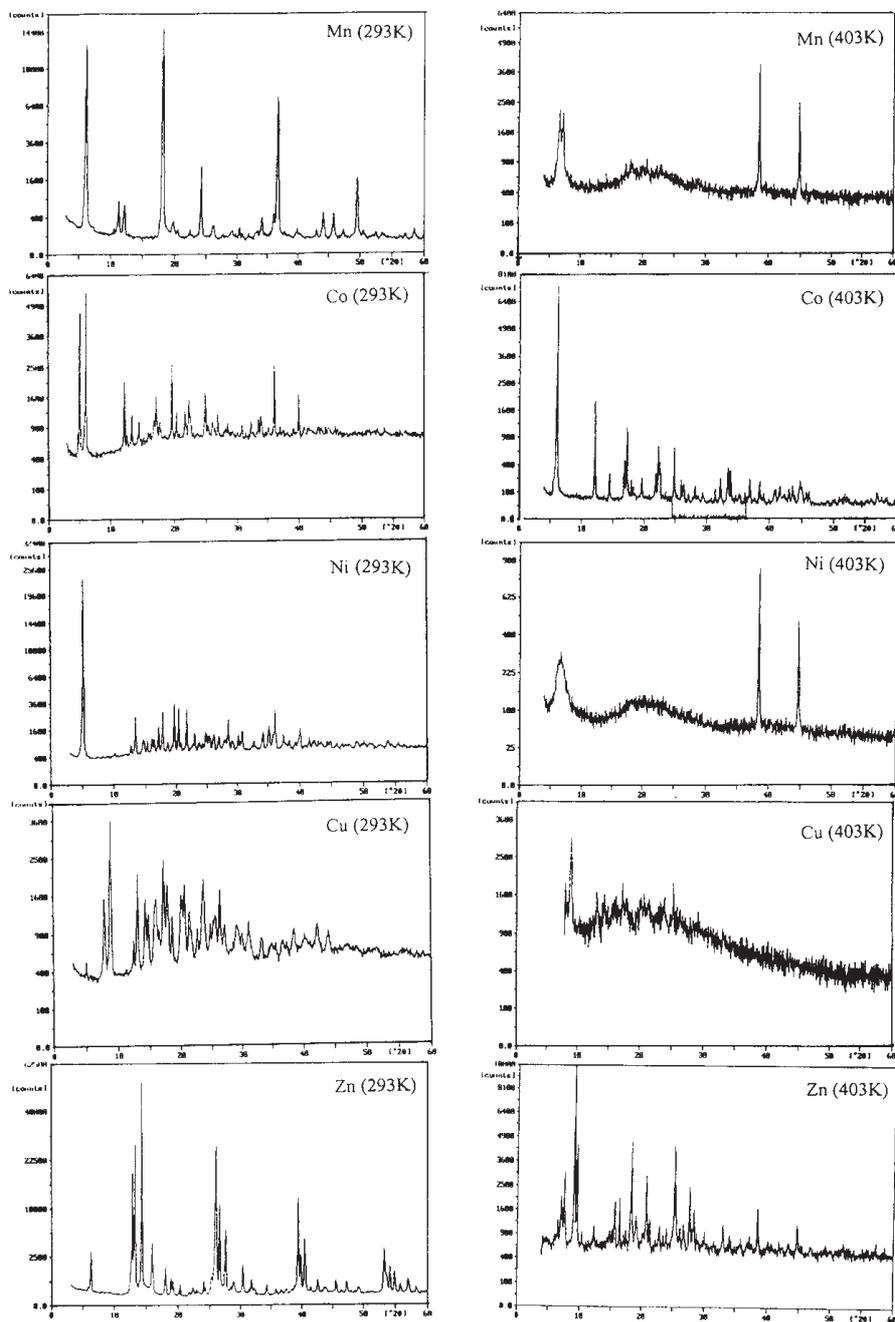
Fig. 3 Diffractograms of 5-chloro-2-methoxybenzoates of Mn(II), Co(II), Ni(II), Cu(II) and Zn(II) at 293 and 403 K
