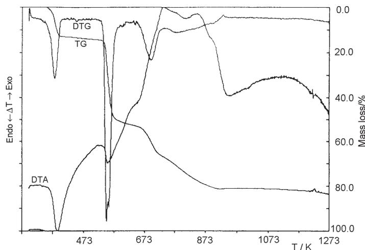
Fig. 4 TG, DTG and DTA curves of 5-chloro-2-methoxybenzoate of Mn(II) in air
