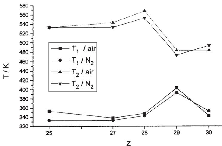
Fig. 5 Relationships between the temperatures of initial dehydration ( $T_1$ ) and decomposition of anhydrous complex ( $T_2$ ) and  $Z$
