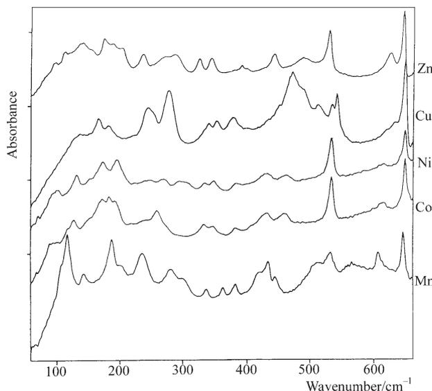
**Fig. 1** Far-infrared spectra of 5-chloro-2-methoxybenzoates of Mn(II), Co(II), Ni(II), Cu(II) and Zn(II)
