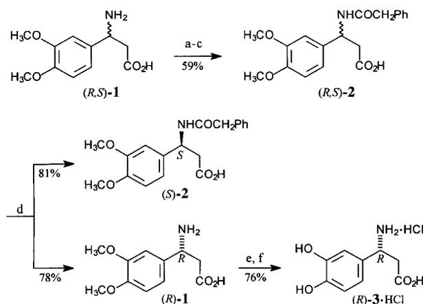
Scheme 1. Synthesis of (*R*)-**3**. a) MeOH, cat. HCl, reflux; b)  $\text{PhCH}_2\text{COCl}$ ,  $\text{CH}_2\text{Cl}_2$ ,  $\text{NEt}_3$ , cat. DMAP; c) LiOH,  $\text{H}_2\text{O}/\text{MeOH}$  (1/1); d) penicillin acylase, pH 7.5, phosphate buffer, 25 °C, 12 h; e) 48% HBr, 145 °C, 4 h; f) Dowex 50 WX8. DMAP = 4-dimethylaminopyridine.
