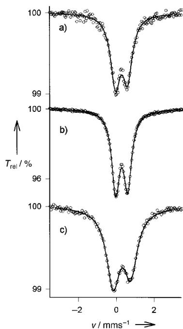
Figure 1. Mössbauer spectra at room temperature. a) Freeze-dried *C. violaceus*; b) water extract; c) synthetic 1:2 iron(III)- $\beta$ -dopa complex at pH 6.2.  $T_{\text{rel}}$  = relative transmission.
