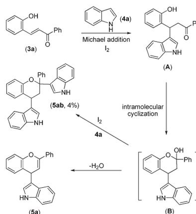
Scheme 5 Proposed mechanism for the domino reaction.
