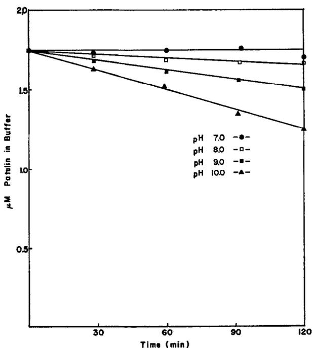
FIG. 6. Stability of Patulin at Various pH's. 0.025 ml of a 10 mg/ml solution of patulin was added to 1.0 ml of 0.1N tris-HCl buffer of different pH's and incubated at 28°C. 0.10 ml of the buffer-patulin solution was assayed at various times by placing it in 2.9 ml of 0.1N HCl in a uv cell. The O.D. at 276 nm was measured and the amount of patulin remaining in the buffer was calculated using 13,350 as the molar extinction coefficient of patulin at 276 nm.
