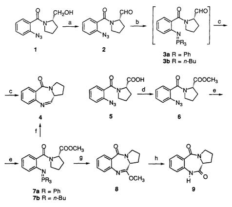
Reagents and conditions: a) PCC,  $CH_2Cl_2$ , r.t., b) TPP,  $Et_2O$ , 0°C (for 3a), or *n*-Bu<sub>3</sub>P,  $Et_2O$ , -10°C (for 3b).c)  $Et_2O$ , r.t. 1 h (for 3a), or  $Et_2O$ , r.t. 30 min (for 3b), d) SOCl<sub>2</sub>, benzene, r.t., then CH<sub>3</sub>OH r.t. e) TPP, CH<sub>2</sub>Cl<sub>2</sub>, r.t.,f) DIBAL,  $Et_2O$ , -78°C  $\rightarrow$  r.t. g) toluene, 140°C sealed tube, 24 h (for 7a), or toluene, reflux, 3 h (for 7b), h) H<sub>2</sub>O, reflux, 30 min.
