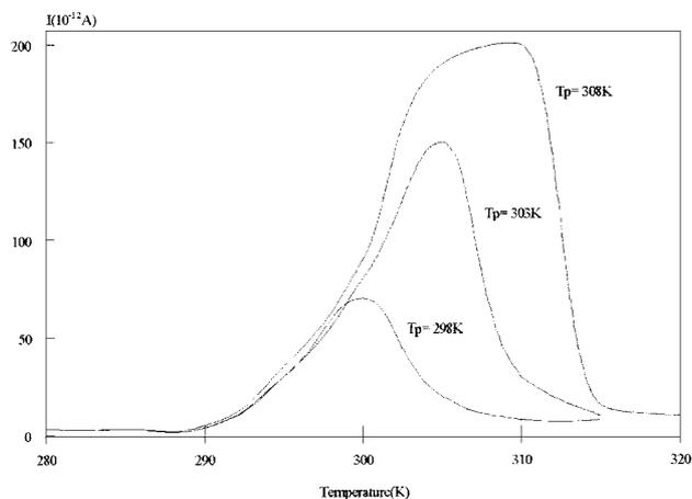
**Figure 3.** Effect of polarizing temperature on peak magnitude of 300K peak.
