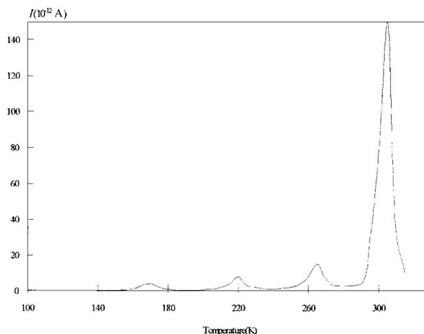
Figure 1. TSDC spectrum of amylase ( $E_p=2$  kV,  $T_p=300$  K,  $h=9\%$ ).
