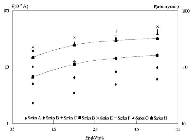
**Figure 2.** Effect of poling field on peak magnitude and stored polarization. (Series A, B, C: peak magnitude ( $I$ ) for 170K, 220K and 265K peaks, respectively. Series E, F, G: stored polarization ( $P$ ) for 170K, 220K and 265K peaks, respectively. Series D, H: peak magnitude ( $I$ ) and stored polarization ( $P$ ) for 300K peak, on  $Y_2$  axis.).
