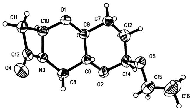
Fig. 1. X-Ray structure of compound **41a** with crystallographical numbering scheme.
