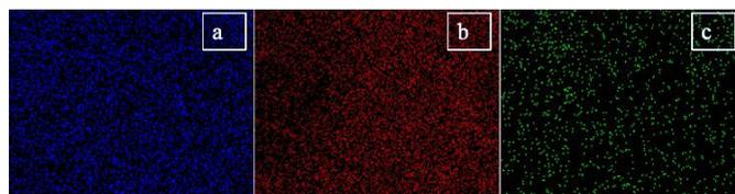
Figure 3. Elemental mapping of Ag/ $\alpha$ -Fe<sub>2</sub>O<sub>3</sub> (a) Fe, (b) O, and (c) Ag.
