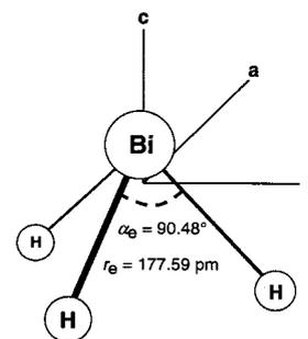
Figure 1. Molecular structure of BiH<sub>3</sub> with principal axes of inertia indicated;  $\alpha_e$ ,  $r_e$  = bond angle and length in the equilibrium structure.
