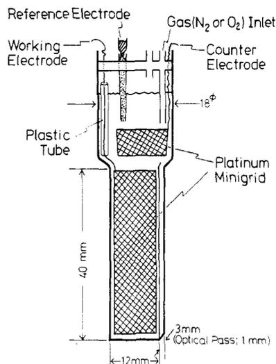
Figure 1. Structure of the OTTLE used.
