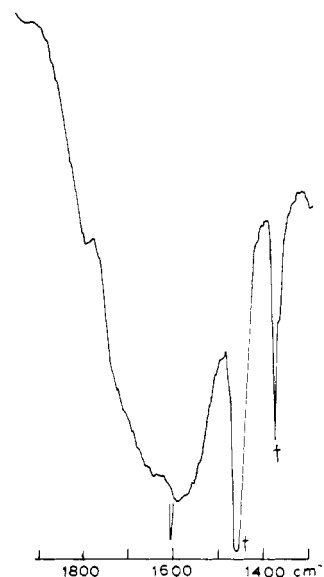
Figure 1. Mineral oil mull infrared spectrum of unsolvated \text{Na}_3[\text{Mn}(\text{CO})_4] in the \nu(\text{CO}) region. Position of bands: 1790 (w), 1600 (vs, br) \text{cm}^{-1} . The daggers show bands due to mineral oil. A polystyrene reference band at 1602 \text{cm}^{-1} is indicated below the most intense carbonyl absorption.
