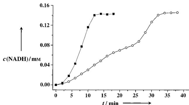
Figure 2. Influence of  $\text{O}_2$  on the indirect electrochemical regeneration of NADH;  $[\text{Cp}^*\text{Rh}(\text{bpy})\text{Cl}]\text{Cl}$  ( $0.1 \text{ mM}$  in  $50 \text{ mM}$  potassium phosphate buffer pH 7.5) (■ no air insertion; ○ air input  $10 \text{ cm}^3 \text{ min}^{-1}$  until  $t = 25 \text{ min}$ ).
