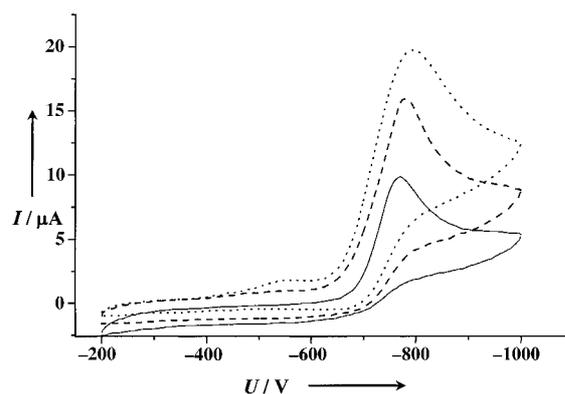
Figure 1. Catalytic effects of  $[\text{Cp}^*\text{Rh}(\text{bpy})\text{Cl}]\text{Cl}$  ( $5 \times 10^{-4} \text{ M}$  in  $0.1 \text{ M}$  TRIS/HCl buffer pH 7.5; TRIS = tris(hydroxymethyl)aminomethane) in the presence of various concentrations of  $\text{NAD}^+$  (0 (—),  $5 \times 10^{-4}$  (---), and  $1 \times 10^{-3} \text{ M}$  (-·-·-));  $v = 81 \text{ mV s}^{-1}$ ; degassed buffers.
