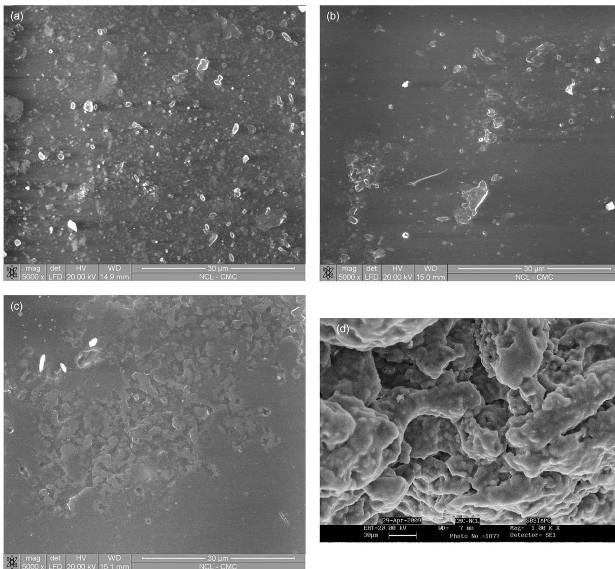
**Fig. 9** (a) SEM micrographs of SBS. (b) SEM micrographs of SBS azide. (c) SEM micrographs of glucose linked SBS. (d) SEM micrographs of tetraacetyl glucose linked SBS.
