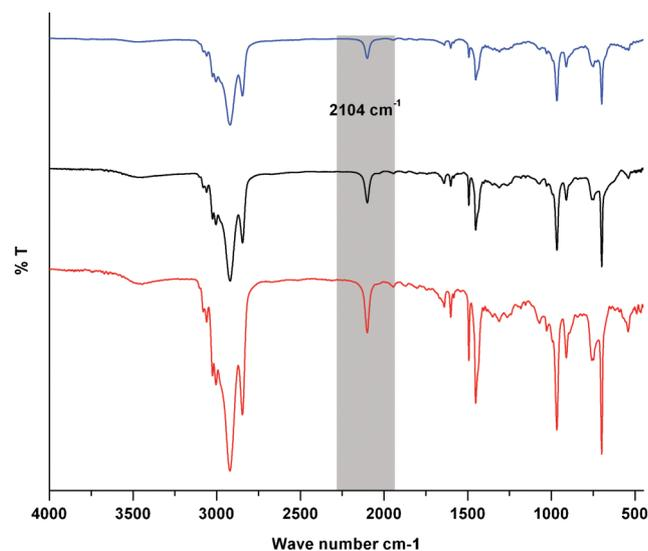
**Fig. 2** SBS azide with different degrees of azidation (increasing intensity of N<sub>3</sub> peak at 2104 cm<sup>-1</sup>).
