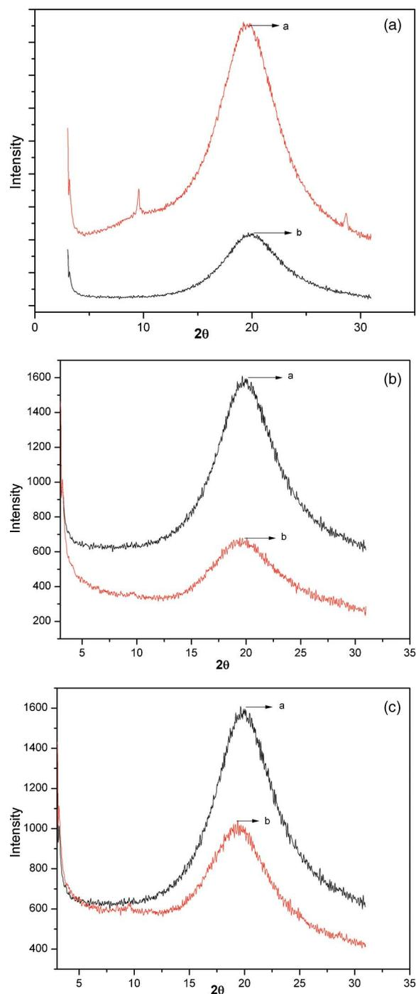
**Fig. 8** (a) WAXRD diffraction plots of curve a (unmodified SBS) and curve b (SBS azide) (b) WAXRD diffraction plots of curve a (SBS azide) and curve b (tetraacetyl glucose linked SBS by click reaction) (c) WAXRD diffraction plots of curve a (SBS azide) and curve b (glucose linked SBS by click reaction).
