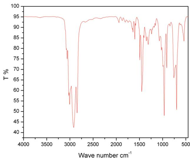
**Fig. 1** FTIR spectra of unmodified SBS.
