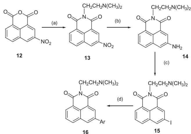
**Scheme 2.** Preparation of 5-arylnaphthalimides. Reagents and conditions: (a) NH<sub>2</sub>(CH<sub>2</sub>)<sub>2</sub>(CH<sub>3</sub>)<sub>2</sub>, EtOH, Δ (67%); (b) HCO<sub>2</sub>H, TEA, Pd/C (100%); (c) NaNO<sub>2</sub>, H<sub>2</sub>SO<sub>4</sub>, KI, 0 °C (44%); (d) ArB(OH)<sub>2</sub>, Pd(PPh<sub>3</sub>)<sub>4</sub>, Na<sub>2</sub>CO<sub>3</sub>, EtOH.
