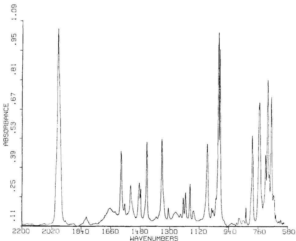
Fig. 1. FTIR spectrum in the  $2200\text{--}600\text{ cm}^{-1}$  region of FeTPP(CO)(py) (CsI pellet; 200 scans;  $0.5\text{ cm}^{-1}$  resolution).
