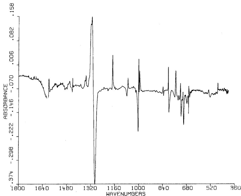
Fig. 8. Difference spectrum obtained by the subtraction of the FTIR spectrum of FeTPP(CS)(EtOH) from that of FeTPP(CS).
