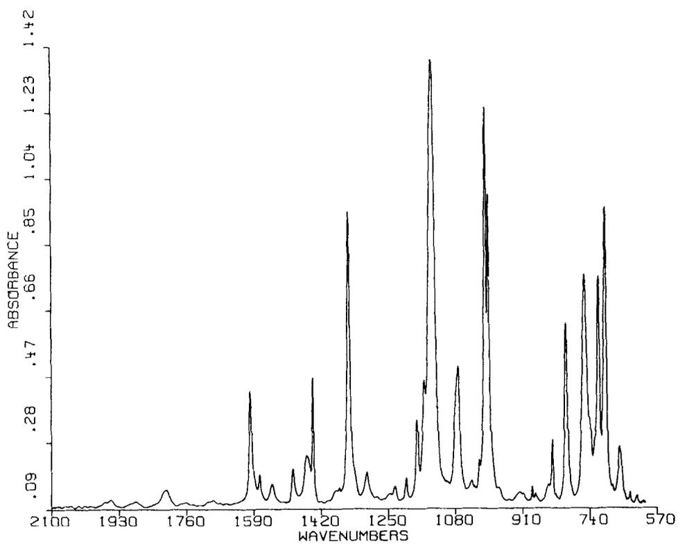
Fig. 3. FTIR spectrum in the 2100–600  $\text{cm}^{-1}$  region of  $\text{FeTPP}(\text{CSe})(\text{EtOH})$  (CsI pellet; 200 scans;  $0.5 \text{ cm}^{-1}$  resolution).
