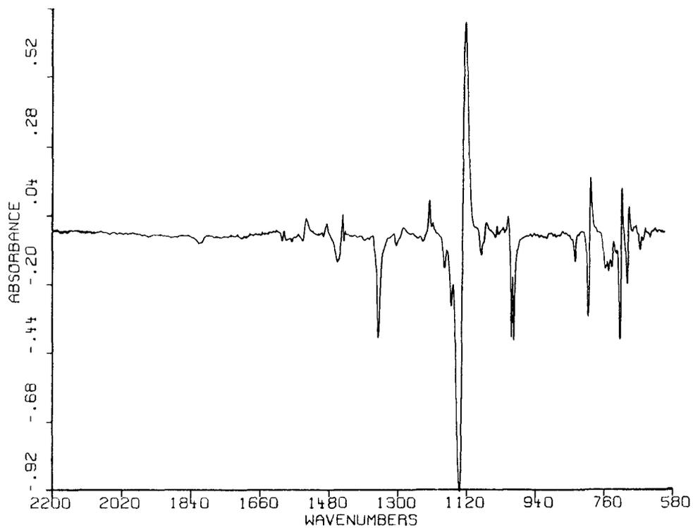
Fig. 7. Difference spectrum obtained by the subtraction of the FTIR spectrum of FeTPP(CSe)(EtOH) from that of FeTPP(CSe)(py).
