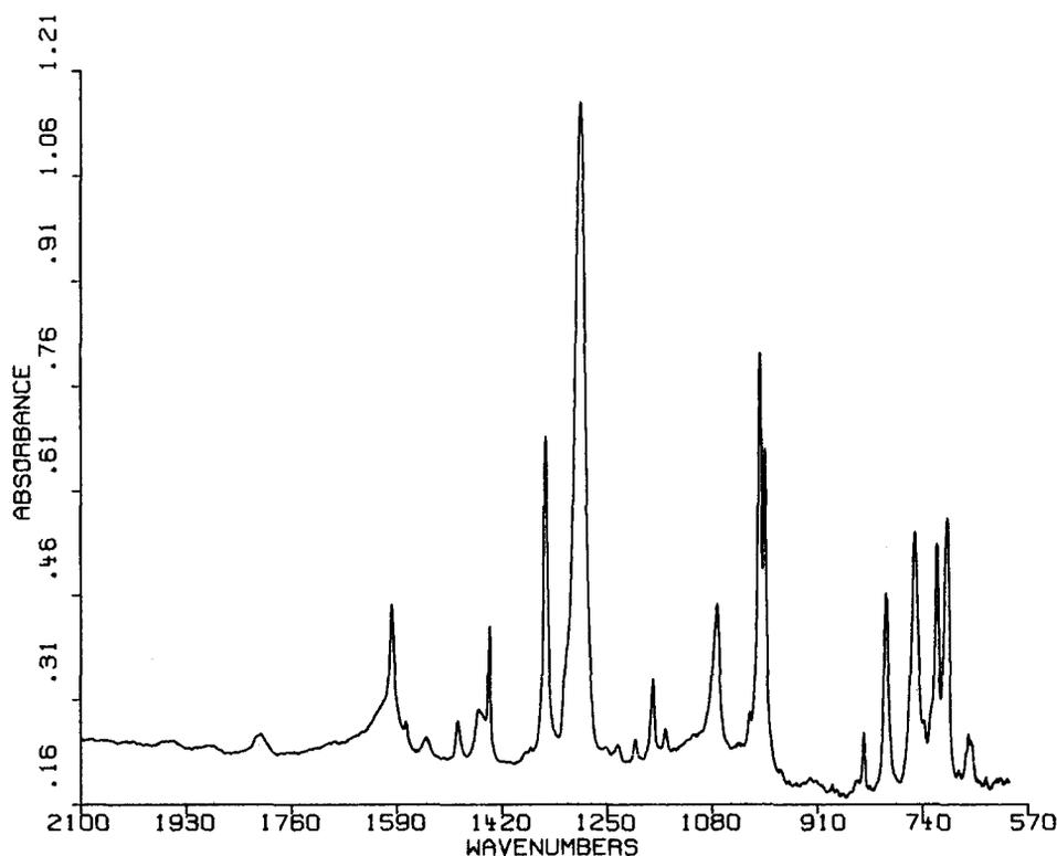
Fig. 2. FTIR spectrum in the 2100–600  $\text{cm}^{-1}$  region of FeTPP(CS)(EtOH) (CsI pellet; 200 scans; 0.5  $\text{cm}^{-1}$  resolution).
