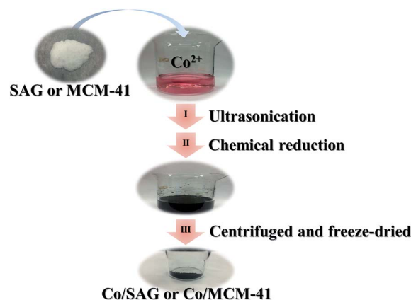
Scheme 1 Illustration of Co-based catalysts synthesis by a facile chemical reduction using \text{NaBH}_4 as reducing agent.
