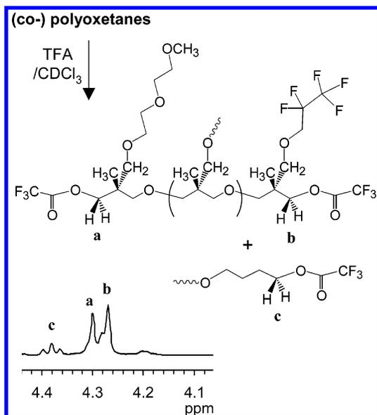
**Figure 3.** Structure and  $^1\text{H}$  NMR spectrum of trifluoroacetyl end groups of copolymers.
