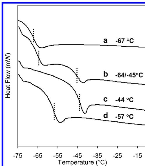
**Figure 8.** Typical DSC curves of polyoxetanes with heating rate of  $20^{\circ}\text{C}/\text{min}$ : (a) ME2Ox homopolymer, (b) physical mixture of ME2Ox and 5FOx homopolymers, (c) 5FOx homopolymer, and (d) ME2Ox/5FOx (1/1) copolymer.
