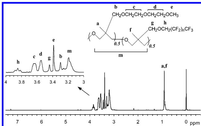
**Figure 2.** Typical  $^1\text{H}$  NMR spectrum of ME2Ox/5FOx (1/1) copolymer.
