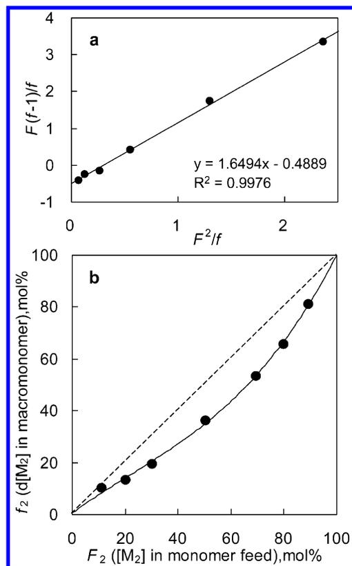
**Figure 6.** F–R plot (a) and composition diagram (b) for ME2Ox/5FOx copolymerization in methylcyclohexane.
