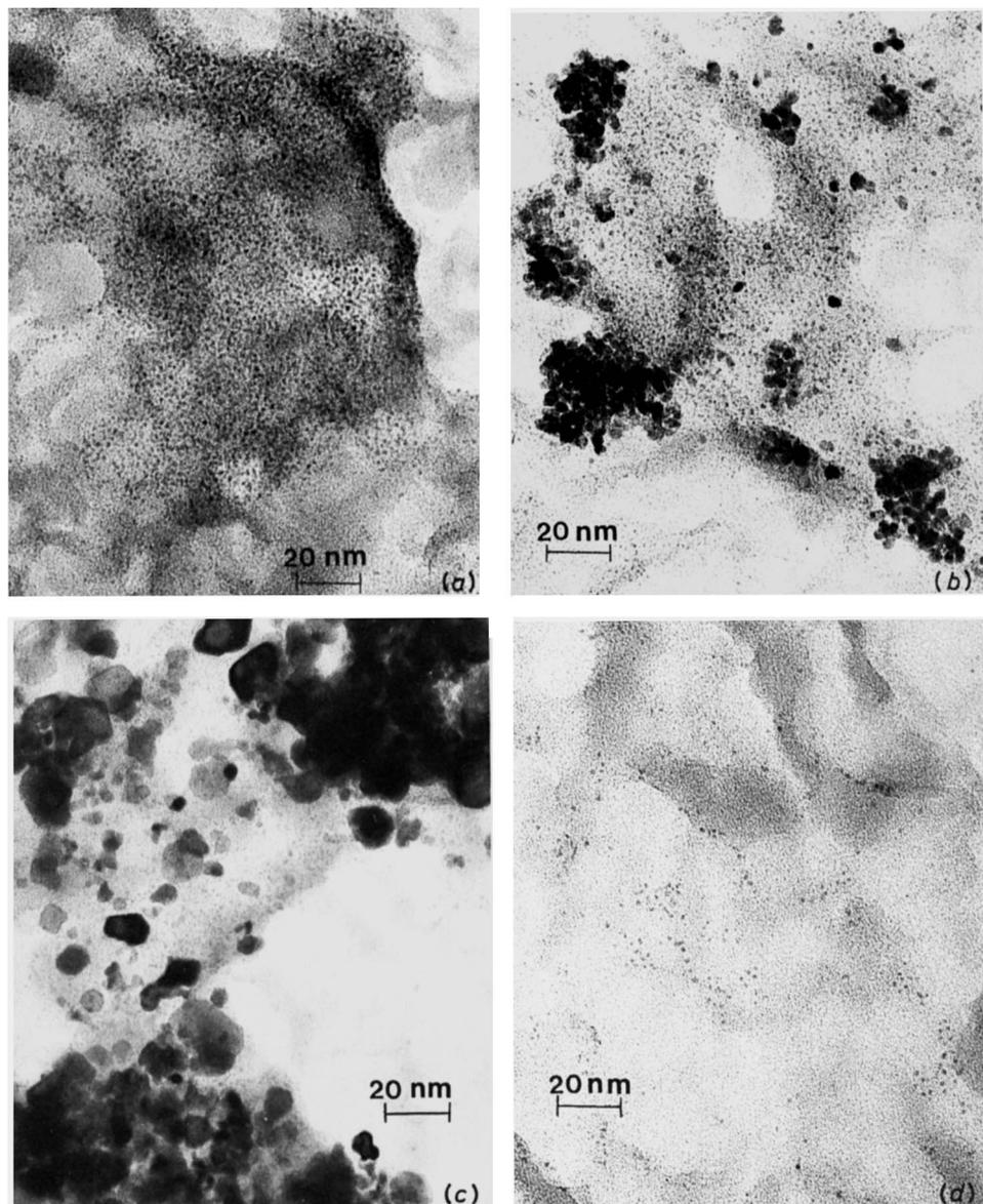
**Plate 1.** Electron transmission micrographs of Pt/Al<sub>2</sub>O<sub>3</sub> catalysts: (a) unchlorinated 1 wt% Pt/Al<sub>2</sub>O<sub>3</sub> sample, (b) 1 wt% Pt/Al<sub>2</sub>O<sub>3</sub> sample chlorinated by CCl<sub>4</sub> at 473 K for 6 h, (c) 1 wt% Pt/Al<sub>2</sub>O<sub>3</sub> sample chlorinated by CCl<sub>4</sub> at 573 K for 0.5 h, (d) 0.1 wt% Pt/Al<sub>2</sub>O<sub>3</sub> sample chlorinated by CCl<sub>4</sub> at 573 K for 0.5 h then reduced at 573 K.
