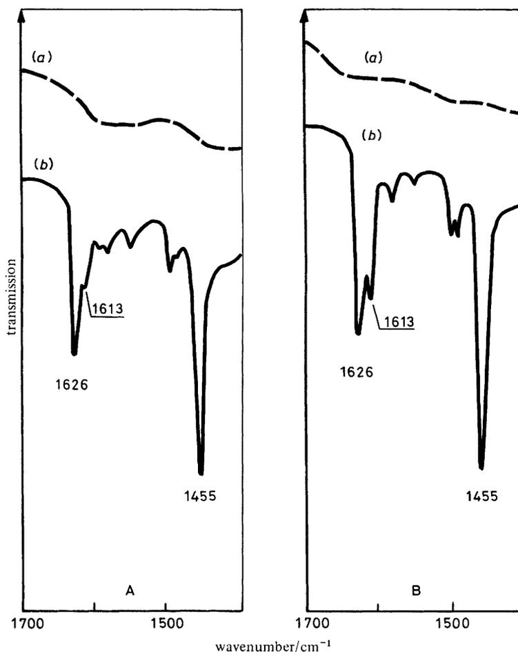
**Fig. 2.** Infrared spectra of pyridine adsorbed on the 5 wt % Pt/Al<sub>2</sub>O<sub>3</sub> sample chlorinated by CCl<sub>4</sub> at 473 K. Chlorination time (A) = 2 h, (B) = 6 h. (a) Chlorinated sample, background; (b) after pyridine adsorption at 300 K and subsequent evacuation at 423 K for several hours.
