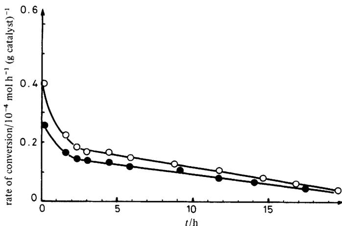
**Fig. 3.** Catalytic activity of the 1 wt% Pt/Al<sub>2</sub>O<sub>3</sub> sample chlorinated by CCl<sub>4</sub> at 473 K for 2 h towards butane conversion: ○, isomerization; ●, Hydrogenolysis. Temperature of reaction = 473 K.
