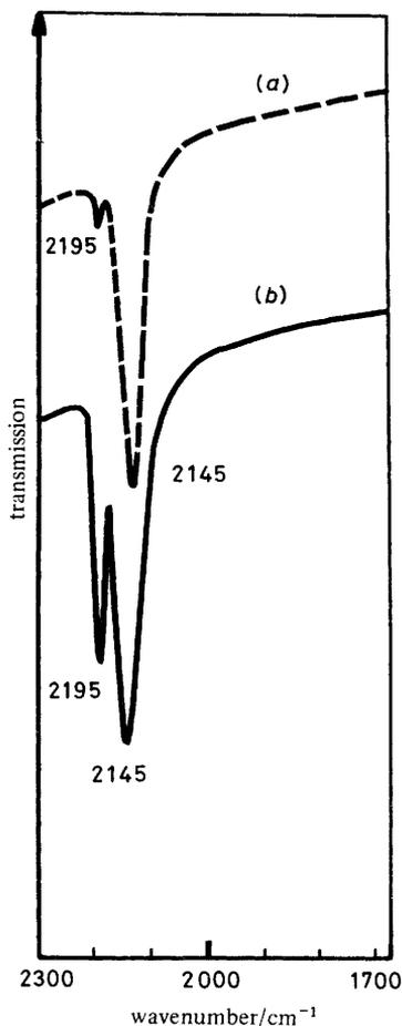
**Fig. 1.** Infrared spectra of carbon monoxide irreversibly adsorbed at 300 K onto the 5 wt % Pt/Al<sub>2</sub>O<sub>3</sub> sample chlorinated at 473 K by CCl<sub>4</sub> (a) for 2 h, (b) for 6 h.
