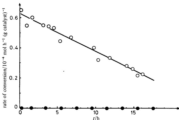
**Fig. 4.** Catalytic activity in n-butane conversion of the 1 wt% Pt/Al<sub>2</sub>O<sub>3</sub> sample chlorinated by CCl<sub>4</sub> at 573 K for 0.5 h: ○, isomerization; ●, hydrogenolysis. Temperature of reaction = 473 K.
