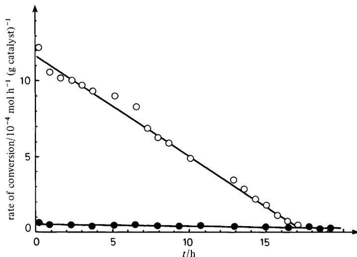
**Fig. 5.** Catalytic activity in n-butane conversion of the 1 wt% Pt/Al<sub>2</sub>O<sub>3</sub> sample chlorinated by CCl<sub>4</sub> at 573 K for 0.5 h: ○, isomerization; ●, hydrogenolysis. Temperature of reaction = 573 K.
