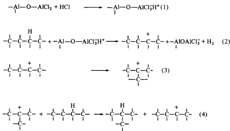
**Scheme 1.** n-Butane isomerization over chlorinated Pt/Al<sub>2</sub>O<sub>3</sub> samples involving the presence of superacid sites. (1) Conversion of Lewis sites into Brönsted centres; (2) hydride abstraction from n-butane; (3) carbocation isomerization; (4) isobutane formation and propagation.
