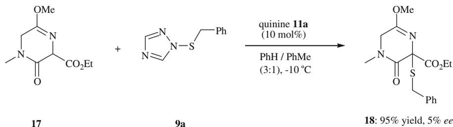
Scheme 3. Organocatalytic  $\alpha$ -sulfonylation of lactim ether **17**.
