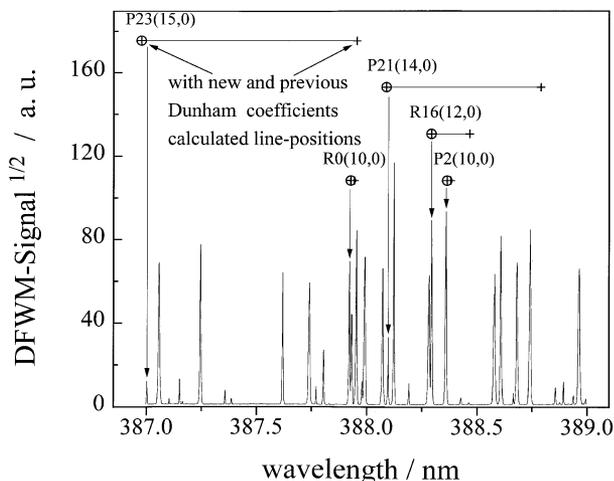
**Fig. 1.** Small part of the DFWM-spectrum of NaH with the assignment of some exemplary lines. The crosses indicate the line positions calculated by Dunham coefficients recommended in [3]. The circles with crosses show the calculated positions if the new set of coefficients for the  $A^1\Sigma^+$ -state given in Table 2 is used. The improvement of the accuracy is obvious especially for high  $J$ -values
