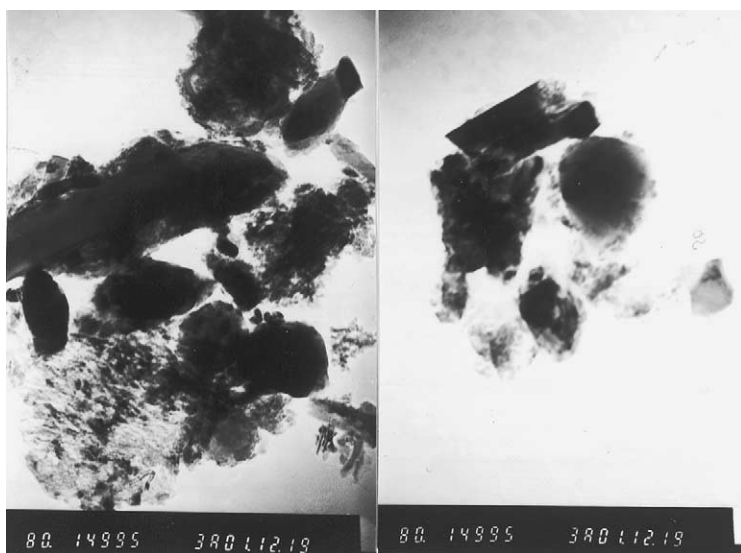
Fig. 3. TEM images of the as-prepared FeP sample (scale bar, 250 nm).
