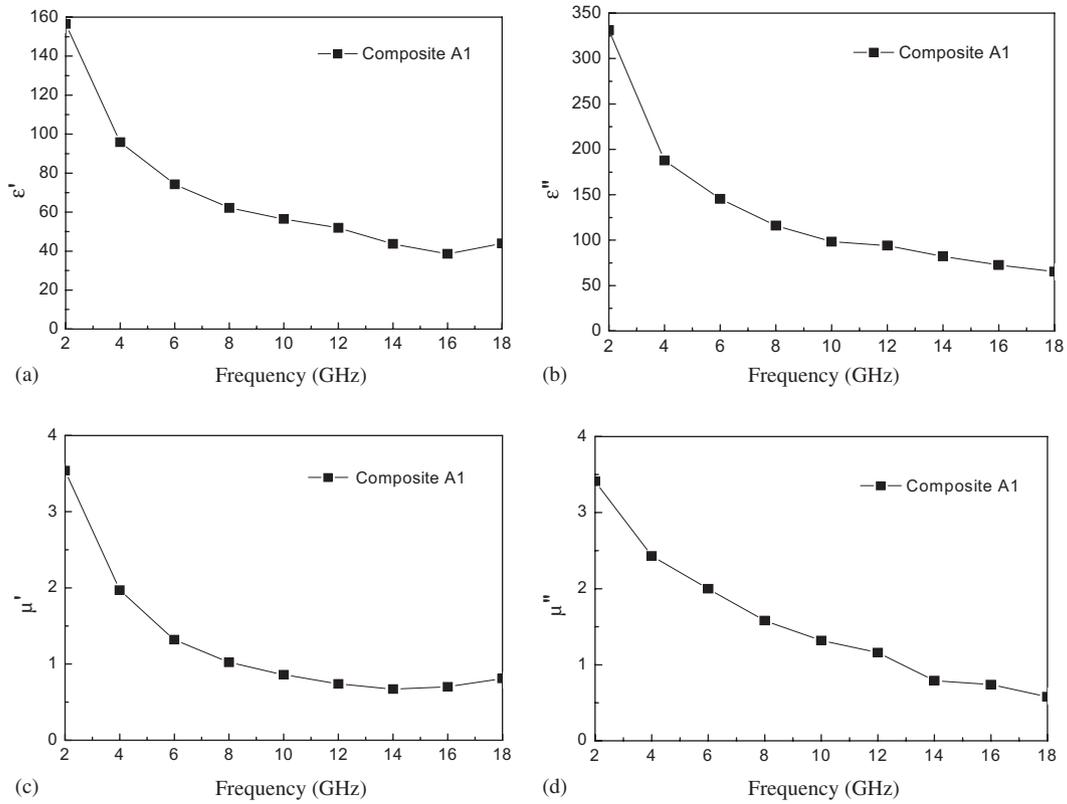
Fig. 4. Complex permittivity and permeability of composites A1 versus frequency: (a) the real part of the permittivity, (b) the imaginary part of the permittivity, (c) the real part of the permeability, and (d) the imaginary part of the permeability.
