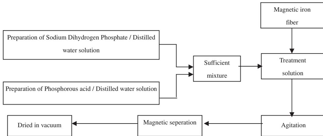
Fig. 2. The phosphating process flow.
