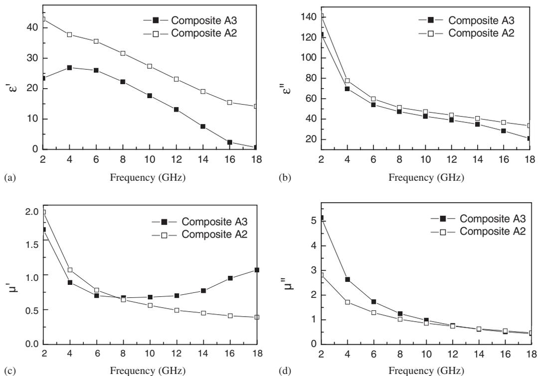
Fig. 5. Complex permittivities and permeabilities of composites A2 and A3 versus frequency: (a) the real part of the permittivity, (b) the imaginary part of the permittivity, (c) the real part of the permeability, and (d) the imaginary part of the permeability.
