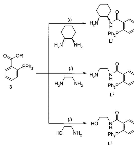
Scheme 1. Synthesis of the Ligands **L**<sup>1</sup>, **L**<sup>2</sup>, and **L**<sup>3</sup>; R = *N*-succinimido; (i) dichloromethane, room temperature
