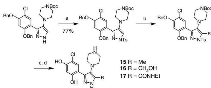
**Scheme 3.** Synthesis of 5-analogues of 3-aryl,4-piperazinyl pyrazoles. Reagents and conditions: (a) TsCl, pyr, CH<sub>2</sub>Cl<sub>2</sub>, rt, o/n; (b) *i*-*n*-BuLi, THF, -78 °C, 10 min; ii—MeI (R = Me) or <sup>t</sup>BuOCOCl (R = CO<sub>2</sub><sup>t</sup>Bu) or EtNCO (R = CONHEt), warm to rt; (c) BCl<sub>3</sub>, CH<sub>2</sub>Cl<sub>2</sub>, 0 °C to rt; (d) (R = CH<sub>2</sub>OH only) LAH, Et<sub>2</sub>O, rt, 2 h.
