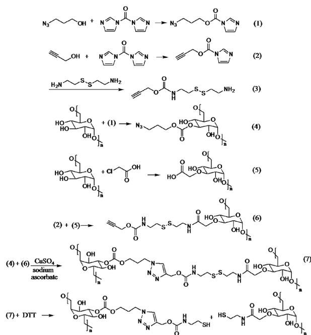
**Scheme 2** The synthesis route to azide-modified dextran (4) and alkyne-modified dextran (6). A click reaction between (4) and (6) crosslinks the dextran chains (7). Cleavage of the disulfide bond by DTT degrades the dextran network and produces free dextran chains.
