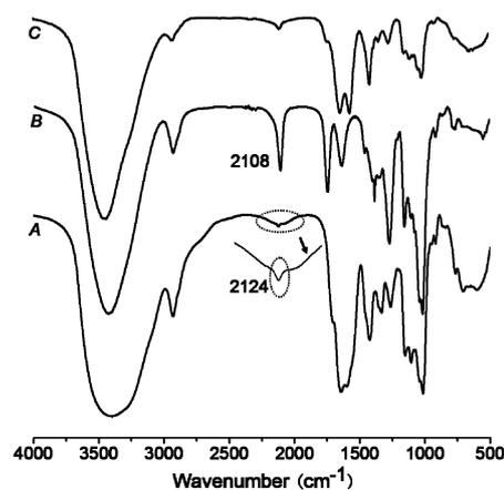
**Fig. 1** FTIR spectra of alkyne-modified dextran (A), azide-modified dextran (B) and a dextran click microgel (C). The extra curve is an expansion of the alkyne stretch shown in curve A.
