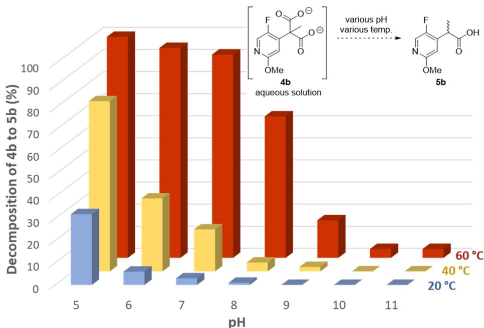
**Figure 5.** Stability profile of an aqueous solution of **4b** at various pH values and temperatures after 7 days showing the percentage decomposition of **4b** to **5b** from spontaneous decarboxylation (for earlier time point data, see the [Supporting Information](#), section 1.4.2).
