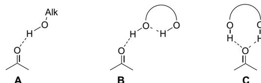
**Figure 1.** Three modes of carbonyl activation by H-bonding: (A) single H-bond activation, (B) single H-bond activation enhanced by intramolecular H-bonding, (cooperative catalysis) (C) double H-bond activation.
