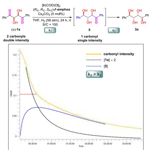
**Scheme 4.** React kinetics obtained with FTIR demonstrating a stepwise pathway. An approximation was made that the intensity of carbonyl peak is proportional to the numbers of carbonyls, regardless of different species. **5** was isolated in 30% yield with 4:1 dr<sup>16</sup> and >99.9% ee (major), and tetraol **3a** was isolated in 62% yield with >99:1 dr and >99.9% ee. Only a trace amount of **1a** was detected.
