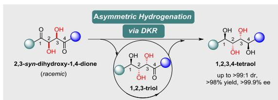
Presented herein is an Ir/*f*-amphox-catalyzed asymmetric hydrogenation of racemic 2,3-*syn*-dihydroxy-1,4-diones *via* dynamic kinetic resolution to produce 1,2,3,4-tetraols. This protocol constitutes an efficient and straightforward approach to accessing chiral sugar alcohols. The nature of the reaction was revealed as a stepwise transformation by *in situ* FTIR spectroscopy and isolation of intermediates.
