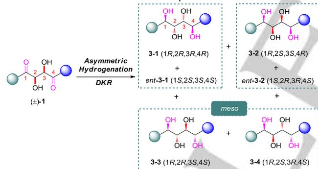
**Scheme 3.** Concept of catalytic asymmetric hydrogenation of 2,3-*syn*-dihydroxy-1,4-diones.
