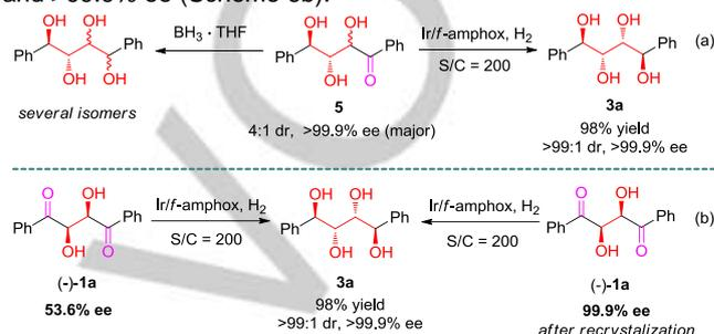
**Scheme 6.** Hydrogenation of optically active triol **5** and diol (-)-**1a**.
