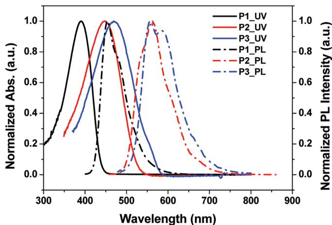
**Figure 2.** UV-vis absorption and PL spectra of the copolymers in the chloroform solution.
