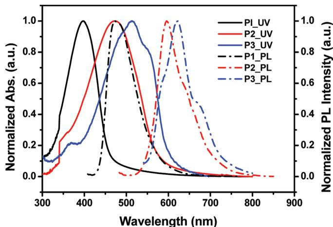
**Figure 3.** UV-vis absorption and PL spectra of P1, P2, and P3 as films.
