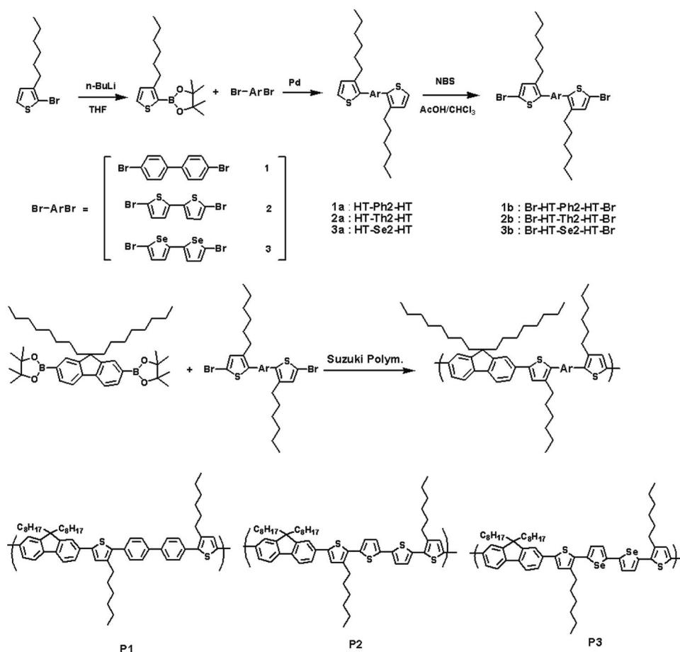
**Scheme 1.** Synthetic scheme for the monomers and copolymers.
