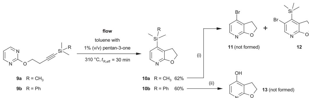
**Scheme 3.** Attempted synthesis of the key building blocks bromo-pyridine **11** and pyridine phenol **13** from dihydro-pyridine model compounds **10a** and **10b**, respectively. Reagents and conditions: (i)  $\text{Br}_2$ ,  $\text{DCM}$ , rt, 3 h, **12**: 43%; (ii)  $\text{H}_2\text{O}_2$ ,  $\text{KHF}_2$ ,  $\text{MeOH}$ , rt, 16 h or  $\text{H}_2\text{O}_2$ ,  $\text{KHF}_2$ ,  $\text{MeOH}$ , 55 °C, 48 h.
