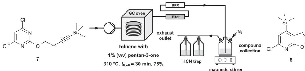
**Scheme 2.** Illustration of the flow reactor configuration that was employed for the previously described synthesis of trimethylsilyl-substituted bicyclic pyridine **8** starting from 2-alkoxy substituted pyrimidine **7**.
