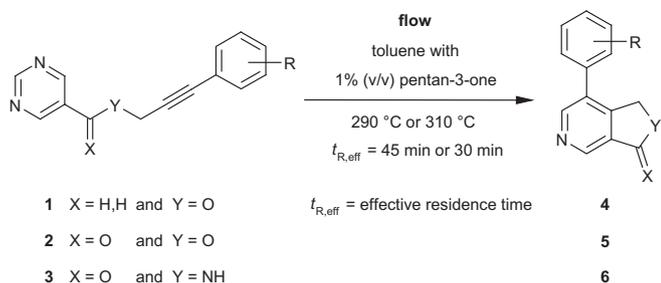
**Scheme 1.** Flow synthesis of 5-aryl-substituted annulated pyridines **4–6**.
