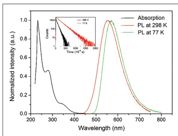
**Figure 2.** Absorption and photoluminescence (PL) spectra of **1**. The inset is the emission decay behavior of **1** in the solid state at 298 and 77 K.
