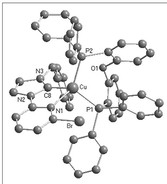
**Figure 1.** X-ray crystal structure of **1**. H atoms, CH<sub>3</sub>COCH<sub>3</sub>, and PF<sub>6</sub><sup>-</sup> are omitted for clarity. Selected bond lengths (Å) and angles (°) are as follows: Cu-N1 2.309(3), Cu-C8 1.964(3), Cu-P1 2.2566(9), Cu-P2 2.2693(10), and N1-Cu-C8 77.55(13), C8-Cu-P1 122.89(10), P1-Cu-P2 114.41(3), and P2-Cu-N1 121.96(8).
