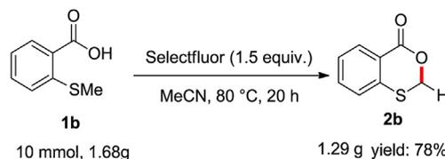
**Scheme 6.** A gram-scale reaction for the synthesis of benzoxathiin-4-one **2b**.
