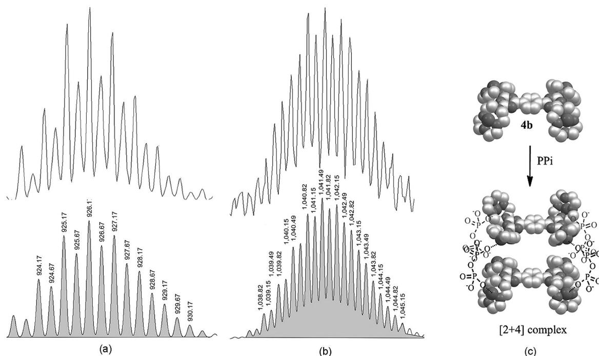
Figure 6. Isotope distribution for ions: (a)  $m/z = 923$   $[(4\mathbf{c} - 4\text{Cl}^- + \text{PPi}^{4-} + \text{Na}^+)_2]^{2+}$ , (b)  $m/z = 1036$   $[(4\mathbf{b} - 8\text{Cl}^- + 2\text{PPi}^{4-} + \text{Na}^+)_2 + \text{Na}^+]^{3+}$ , and (c) proposed structure of dimer  $[4\mathbf{b} - 8\text{Cl}^- + 2\text{PPi}^{4-}]_2$ .
