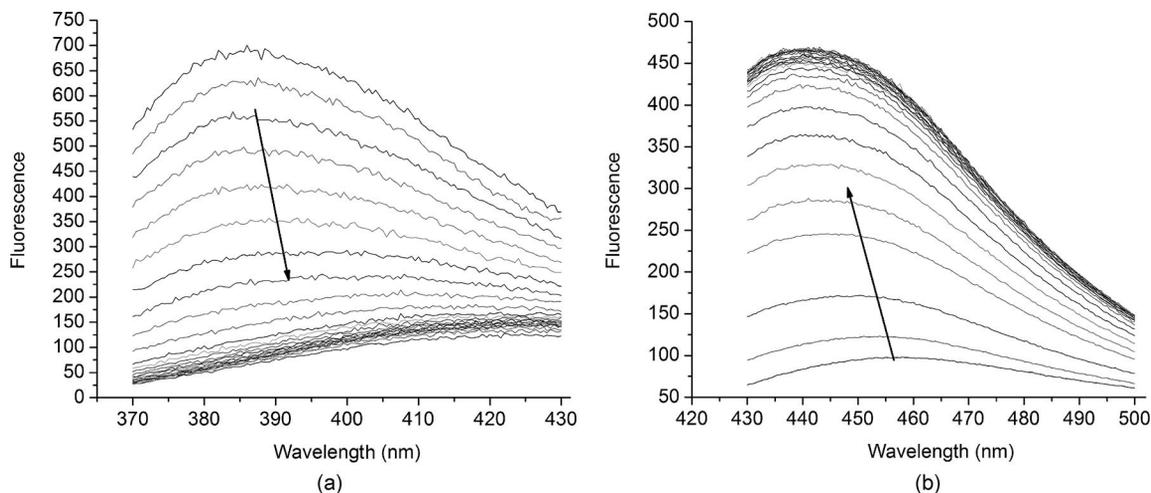
Figure 5. Fluorescence response upon addition of sodium pyrophosphate to the solution of (a) complex **4b** and solution of (b) complex **4d**. Titrations were carried out in 25 mM HEPES buffer, pH 7.4, 25 °C.
