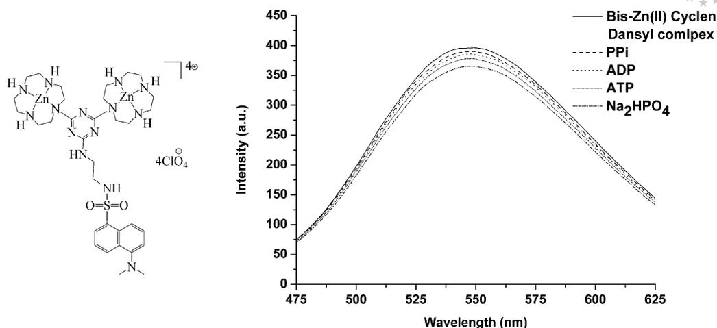
Figure 4. Dinuclear Zn<sup>II</sup>-cyclen dansyl complex with flexible linker between receptor and fluorophore (left); emission intensity changes of binuclear Zn<sup>II</sup>-cyclen dansyl complex (80 μM in HEPES buffer, pH 7.4, λ<sub>ex</sub> = 330 nm, 25 °C) upon addition of various nucleotides and phosphates (right).
