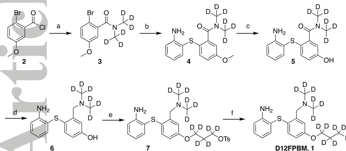
Scheme 1. Reagents and conditions: (a) Dimethyl-d<sub>6</sub>-amine hydrochloride, Et<sub>3</sub>N, DCM, 0 °C to RT, 5 h. (b) Cu, Cu<sub>2</sub>O, 2-aminothiophenol, Et<sub>3</sub>N, 2-ethoxyethanol, 130 °C for 50 h. (c) 1M BBr<sub>3</sub>, DCM, 0 °C to RT, over night. (d) 1M BH<sub>3</sub> in THF, THF, reflux, 8 h. (e) K<sub>2</sub>CO<sub>3</sub>, DMF, [1,1,2,2,3,3-D<sub>6</sub>]-propane-1,3-diylbis(4-methylbenzenesulfonate), 65 °C, 3 h. (f) 1M TBAF in THF, THF, 65 °C, 3 h.
