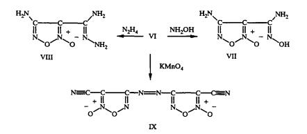
The aminofuroxan (VI) is oxidized by potassium permanganate in an acidic medium to the azo derivative (IX).
