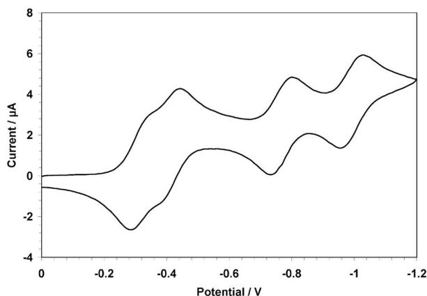
Figure 6. Cyclic voltammograms for the reduction of **11** (1 mM) in benzonitrile containing  $\text{Et}_4\text{NClO}_4$  (0.1 M) as a supporting electrolyte; scan rate:  $100 \text{ mV s}^{-1}$ .
