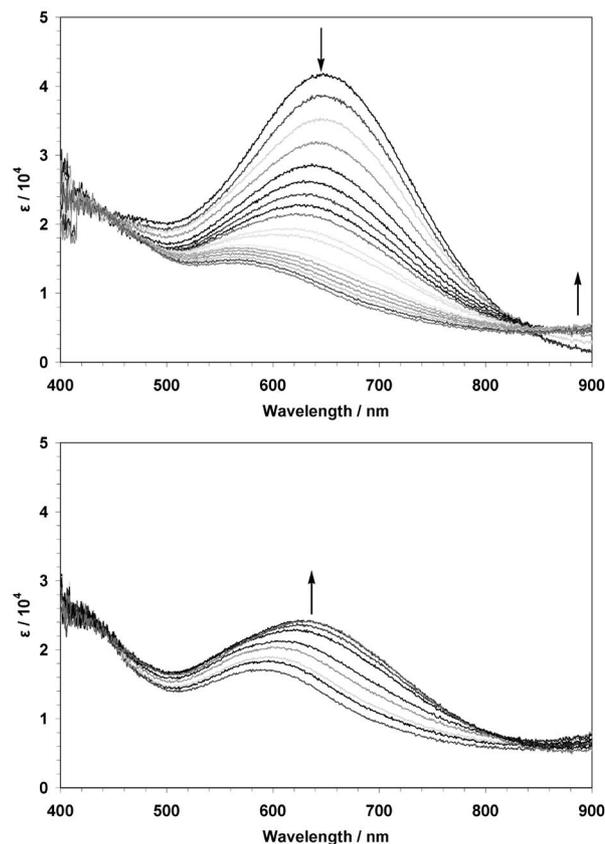
Figure 7. Continuous change in visible spectra of **7** in benzonitrile containing  $\text{Et}_4\text{NClO}_4$  (0.1 M): constant-current electrochemical reduction (50  $\mu\text{A}$ ) at 30 sec intervals (top) and reverse oxidation (bottom) of the reduced species (50  $\mu\text{A}$ ) at 30 sec intervals.
