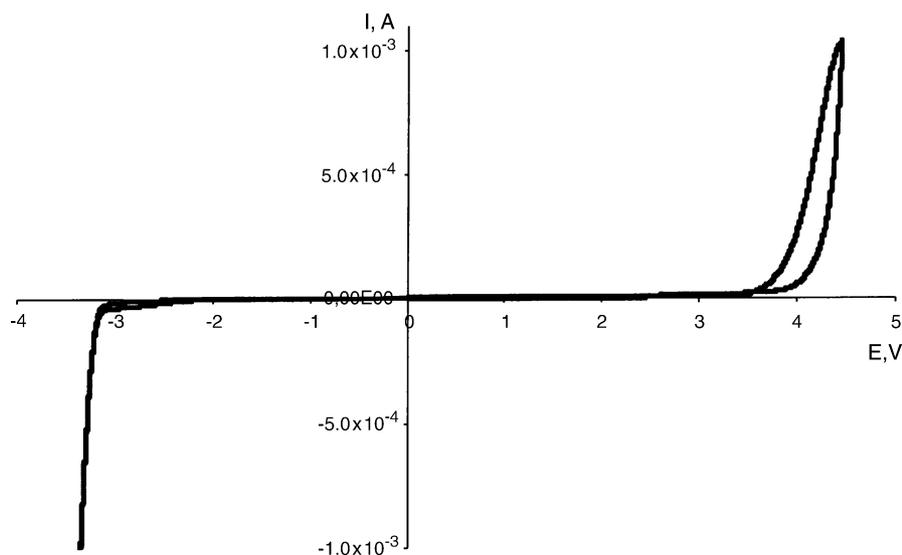
Fig. 2. CVA of tetrabutylammonium tris(pentafluoroethyl)trifluorophosphate.
