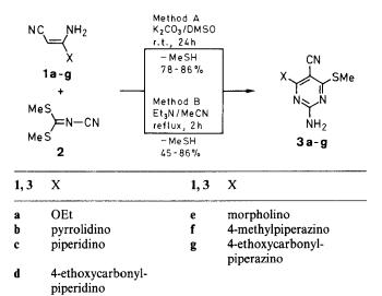
(Method B) the enaminonitriles 1 and compound 2 in a 1:1.5 molar ratio are heated under reflux in acetonitrile in the presence of an excess of triethylamine for a few hours.
