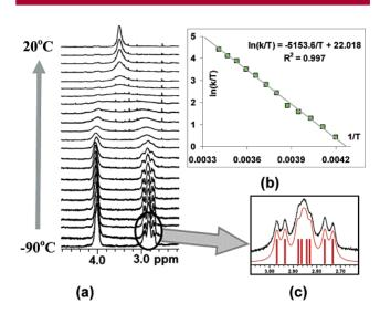
**Figure 4.** (a) VT-NMR for **5f**: 20 to -90 °C at  $\Delta T = 5^\circ$ , CD<sub>2</sub>-Cl<sub>2</sub>. (b) Eyring plot and (c) a 2.8 ppm multiplet (black) simulated with two pairs of doublets (J = 14.1 Hz) with equal intensity (red).
