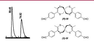
Figure 1. HPLC trace for enantioseparation of **5f** on a Chiralcel OD chiral chromatography column.
